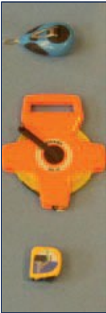
Chalk liner, tape measurement
